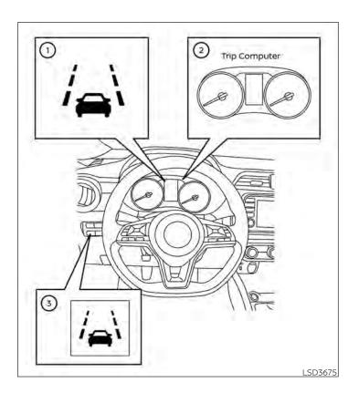
The LDW system provides a lane departure warning function when the vehicle is driven at speeds of approximately 37 mph (60 km/h) and above and the lane markings are clear. When the vehicle approaches either the left or the right side of the traveling lane, the steering wheel will vibrate and the LDW indicator (if so equipped) on the instrument panel will blink to alert the driver.
