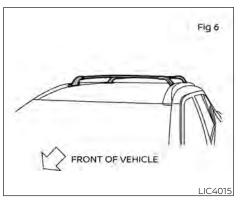
6. Tighten all 4 bolts to 8-9 N-m torque using a T-30 TORX® torque wrench.
