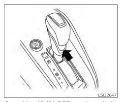
Overdrive (O/D) OFF mode switch (if so equipped)
