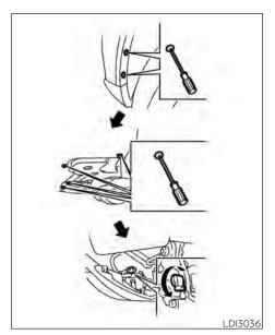
Replacing the fog light bulb (if so equipped)
