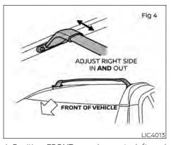
4. Position FRONT crossbar onto left and right roof rack rail; and adjust right support in and out until it fits securely into position. See Fig. 4.
