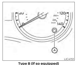
Turn the control knob (A) to adjust the brightness of instrument panel lights.
