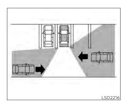
The RCTA system uses radar sensors ① installed on both sides near the rear bumper to detect an approaching vehicle.
