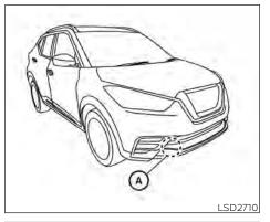
The I-FCW system can help alert the driver when there is a sudden braking of a second vehicle traveling in front of the vehicle ahead in the same lane.
