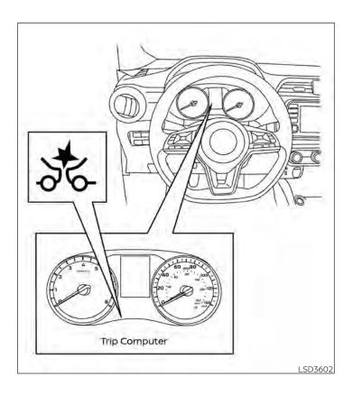
The AEB system warning light (orange) will illuminate and the "Front Radar Obstruction" warning message will appear in the vehicle information display (if so equipped).
