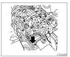
**HR16DE** engine **ENGINE SERIAL NUMBER**
