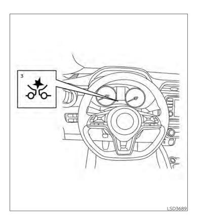
If the driver does not take action, the AEB with Pedestrian Detection system issues the second visual (flashing) (red and white) in the vehicle information display (if so equipped) and an audible warning. If the driver releases the accelerator pedal, then the system applies partial braking. If the risk of a collision becomes imminent, the AEB with Pedestrian Detection system applies harder braking automatically.
