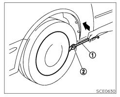
Removing wheel cover (if so equipped)
