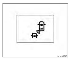
The Blind Spot Warning (BSW) switch is used to turn on and off the BSW system. When the BSW switch is pushed, the BSW system will turn on and the BSW indicator light in the meter will illuminate. When the BSW switch is pushed again, the BSW system will turn off and the BSW indicator light will turn off
